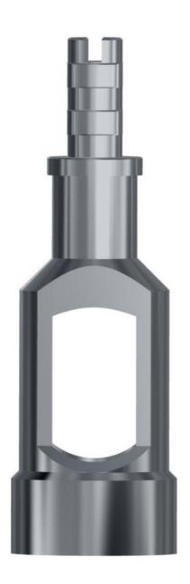
The RMZ Wireline Gauge Cutter is predominantly used for drifting the tubing string but also designed to remove scale, debris, paraffin wax etc. this will ensure that down hole tools will pass through tubing and nipples without obstruction during wireline operations.
