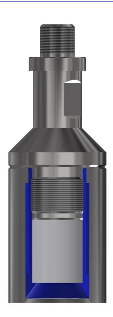
The RMZ Wireline Magnet is a special purpose wireline tool that is used to retrieve small magnetically attractable items such as nuts, bolts, tool parts and any ferrous debris lost within the well bore. The outer sleeve prevents debris from becoming dislodged on retrieval
