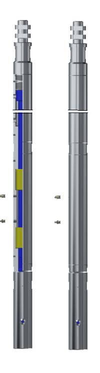
The RMZ Wireline Tubular Linear Jar is a telescoping jar that should be run in conjunction with wireline stem installed immediately above. The linear bearings create a frictionless action, allowing full force of impact from the stem above. The Tubular Linear jar is the ideal tool for use is deviated wells. This tool has a proven record of success in wells with 65-75 degrees deviation.
